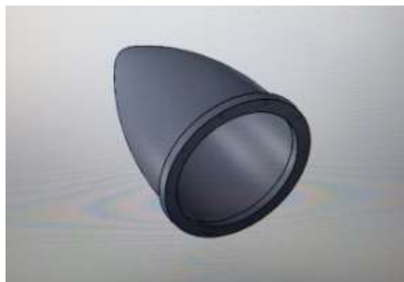
Figure 2: Model of parabolic radome
